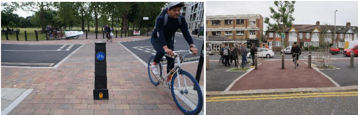
Figure 6-8: Combined informal crossing and modal filter (Downs Road, Hackney), and Modal Filter installed with cycle access (Grove Road, LB Waltham Forest)
